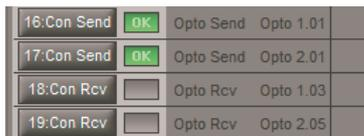
A dual loop console can have 2 snd ports (one per loop) and upto 8 Rcv ports (4 per loop). Console Snd/Rcv ports will use up some of your 1008 optocore channels and also Engine input and output resources.
