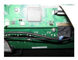
Note mixers have a jumper on CN2 on the right hand section. This is required and affect LED but not motor or control operation if not present.
