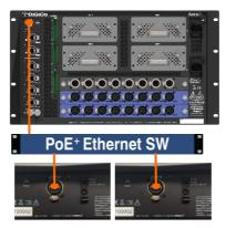
Power up the A-CONTROL8 by plugging the external PSU into the DC In socket or connecting using a CAT5 cable to a PoE+ switch. The port Lnk/Err indicator flashes at a steady rate when the link is established. The unit Name and IP address are displayed on the LCD Displays for easy identification of the unit. After a few seconds the A-CONTROL8 will display the assignments and functions if any have been set for the unit.
