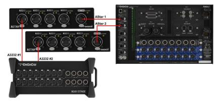
Up to 4 expanders can be connected redundantly to a pair of AStars.
